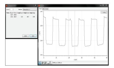
11. Once the calibration software is completely filled out, select Calculate to obtain the new calibration values. Enter these values in the System tab and click Save.
