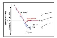
What is actually measured is the deflection of the cantilever, or the Top - Bottom (T-B) signal of the photo-detector.
