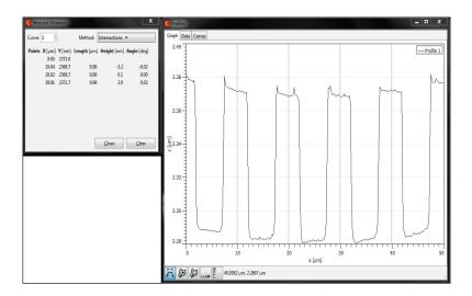
Insert the values in the Length column into each X Measures blanks in the calibration software.
