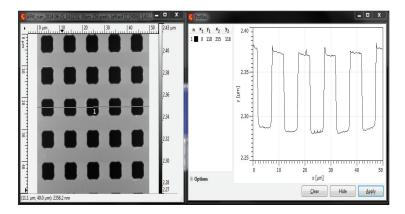
7. Using the Measure Distances feature on the bottom left-hand corner of the extracted profile, create vertical lines that bisect each square at approximately the same poin
