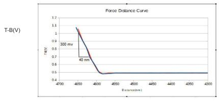
Slope=300mv/40nm = 7.5 mv/nm
