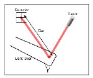
The deflection of the cantilever can be converted to Force using Hook's law:
